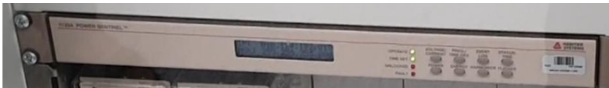
Slika 13: Merilnik fazorjev Arbiter Systems, Model 1133A Power Sentinel
